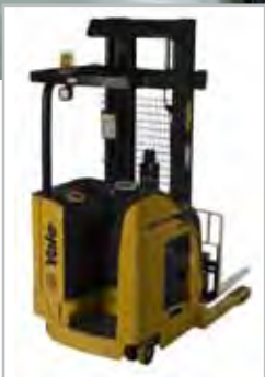
Narrow aisle truck
