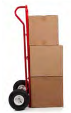
A two-wheel dolly is used to move small volumes of boxed materials
