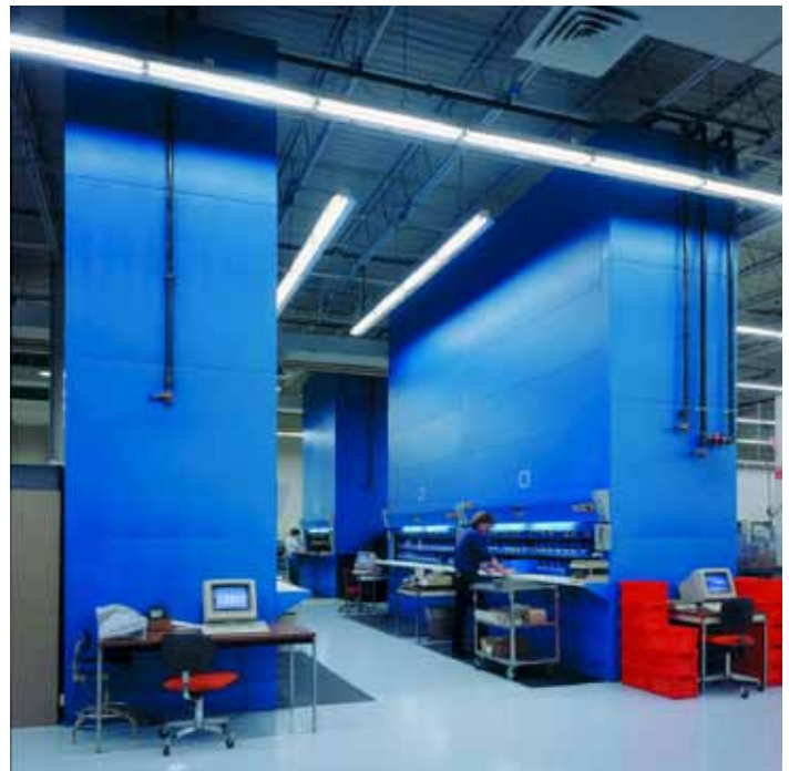
This is a vertical carousel with bins for small parts that rotate vertically to bring the correct items to the level of the order picker.
