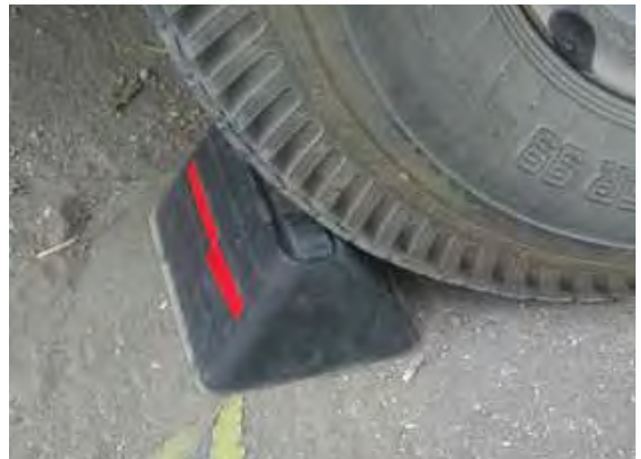
Wheel chocks are used to help ensure that a trailer doesn't move during unloading.
