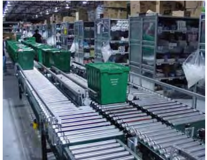
Pick and pass: workers pick items from shelves and pass them into bins on the conveyor.
