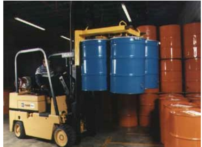
This fork truck has a special attachment to carry barrels and drums
