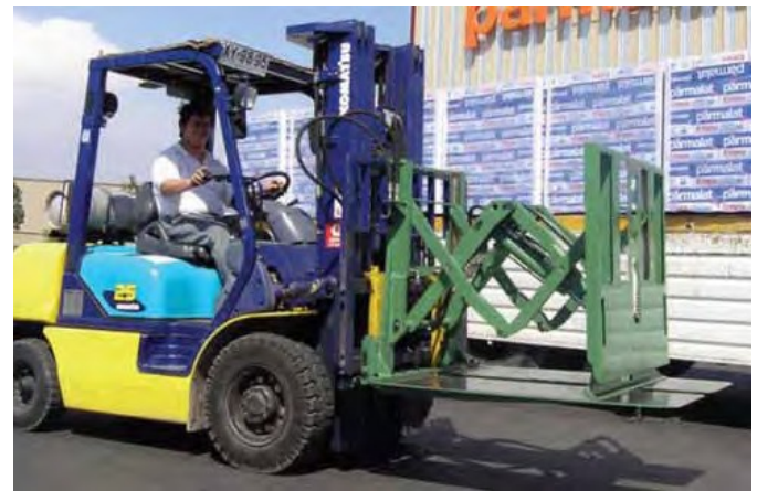
This fork truck has a special slip sheet attachment
