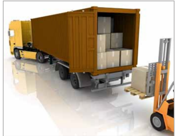
These boxes have been floor loaded.
