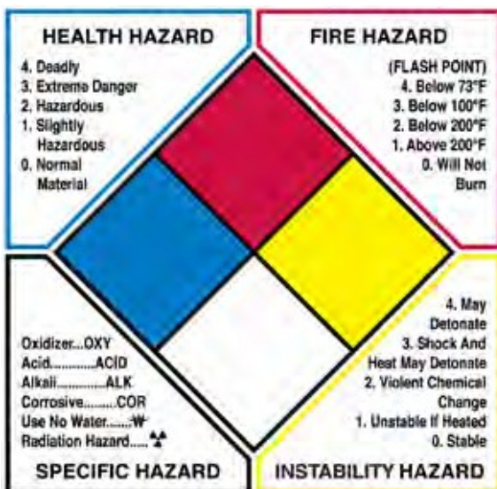
This is the standard format for a hazmat label which may appear on a shipping container or a storage door
