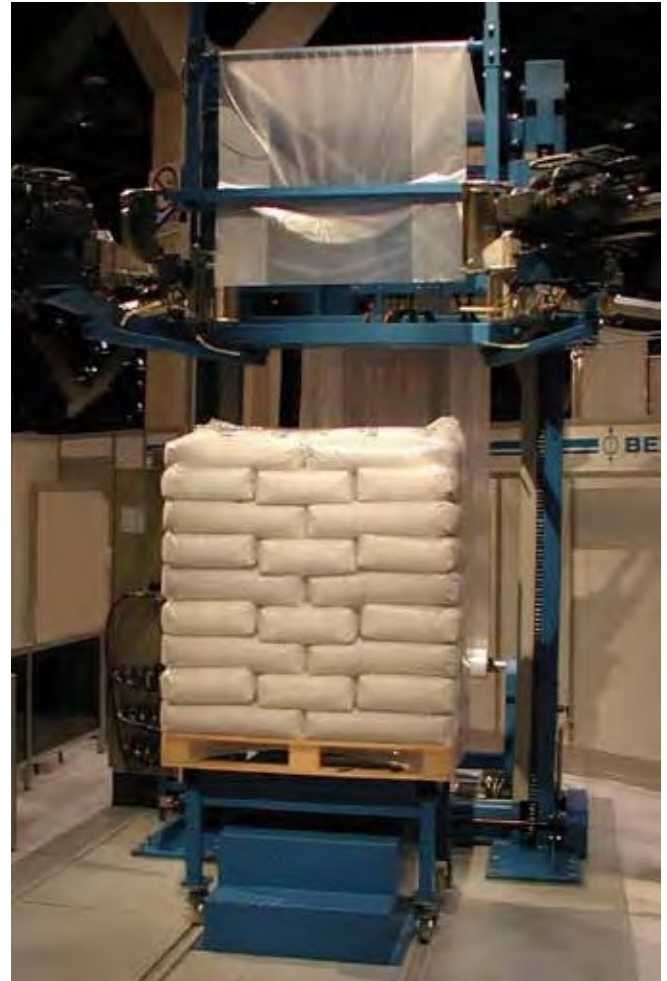
A fully-automated stretch wrapper.
