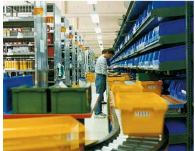
Notice the two types of shelving, standard steel shelves on the left and bin shelving on the right.
