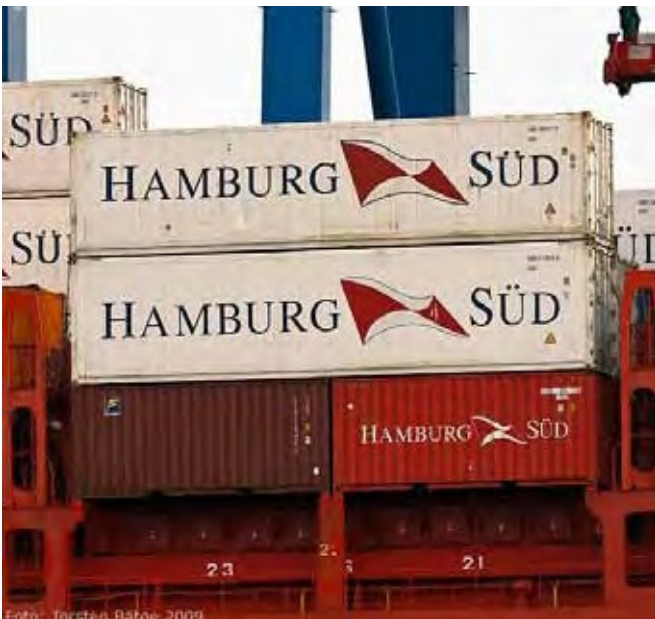
Notice the two intermodal containers on the bottom are 20-feet, while the two white containers are 40-feet
