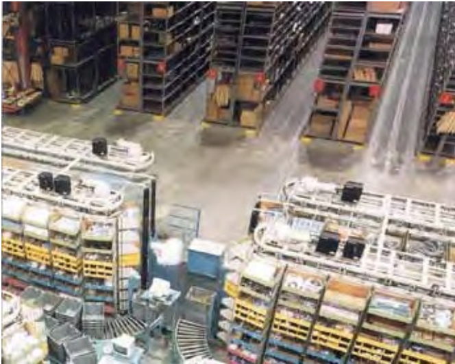
The horizontal carousel moves the bins around so workers can stand in one area and pick multiple SKUs.
