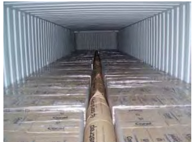
These are inflatable dunnage bags that help keep the cases from shifting during transport.
