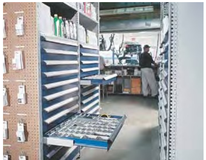
Drawer storage is usually used for small parts like individual nuts and bolts or expensive items like jewelry
