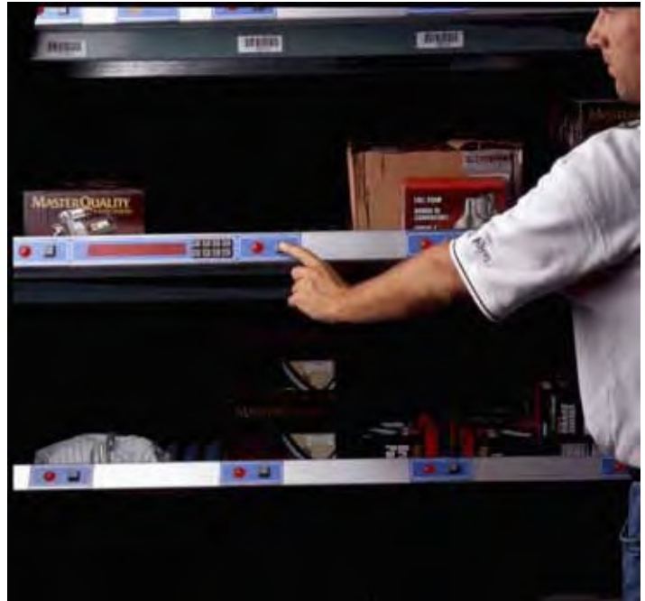
Example of a pick to light system.
